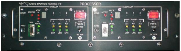
Redundant Control Processor
