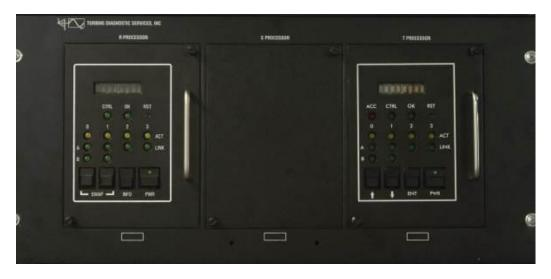
Triple Modular Redundant Processor Chassis
