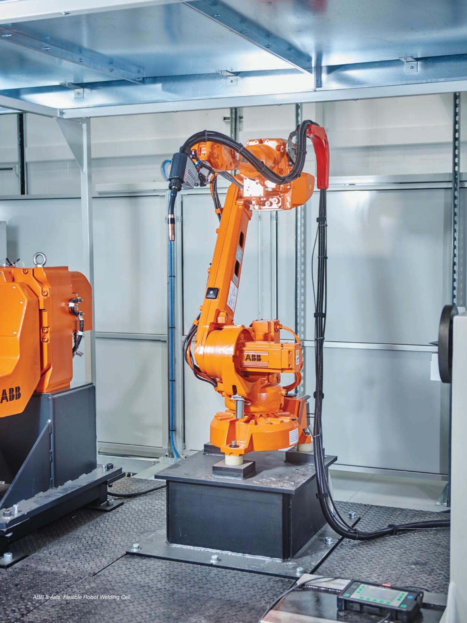
ABB 8 Axis\* Flexible Robot Welding Cell
