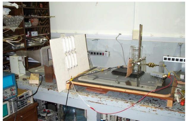
Fig. 8. Is a photograph of the lab setup showing the built plasma dipole FSS with the horn receiver antenna.
