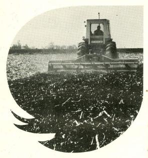
Rotavation is a proven, tested method of complete tillage. Power is taken directly from the tractor PTO and applied directly to the soil working blades. No additional wheel weights or loaded tires are required, since thrust of the power driven blades actually helps propel the tractor forward, eliminating wheel slippage and reducing compaction.
