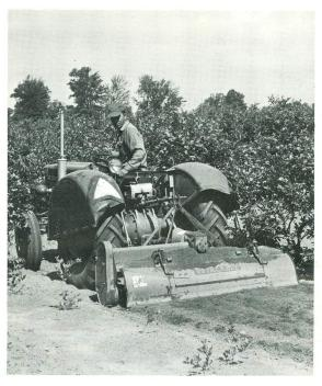
ROTACADET 70" FOR TRACTORS UP TO 45 B.H.P. 70" TILLAGE WIDTH CENTRALLY MOUNTED 540 P.T.O. ONLY WITH TWO SPEED ROTOR STANDARD MODEL C/W TWO DEPTH SKIDS CULTIVATING MODEL C/W TWO DEPTH WHEELS DEPTH WHEELS AVAILABLE AS OPTIONAL EXTRAS
