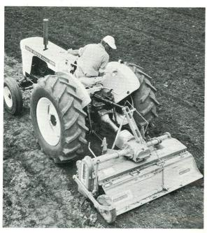
MODEL 'E' 35 TO 60 B.H.P. **OR 3-PLOW TRACTOR POWER** 50", 60", 70" AND 80" TILLAGE WIDTHS 3-POINT MOUNTED OR FAST HITCH 540 OR 1000 P.T.O. WITH MULTI-SPEED ROTOR THROUGH SELECTATILTH GEARBOX
