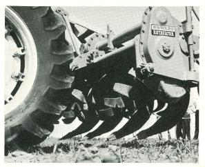
THE ALL NEW ROTACHISEL FROM HOWARD . . . COMBINES THE WORK OF 4 IMPLEMENTS IN ONE; THE PLOW, DISC, HARROW AND THE CHISEL, BREAKS HARDPAN WHILE PREPARING TOPSOIL PREPARES A PERFECT. WELL DRAINED SEEDBED. CHISELS ADJUSTABLE FROM 4" TO 8" BELOW ROTAVATOR BLADES. AVAILABLE IN VARIOUS MODELS AND SIZES.
