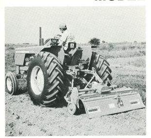
MODEL 'P' FOR 18 TO 40 B.H.P. ON 2 TO 3 PLOW TRACTOR POWER 40", 50", 60" AND 70" TILLAGE WIDTHS WITH SPECIAL OFFSET (PG & P.U.T. MODELS) FOR ORCHARDS AND GROVES. 540 P.T.O. ONLY WITH MULTI-SPEED ROTOR THROUGH SELECTATILTH GEARBOX
