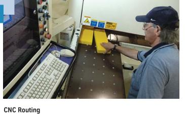
Our dual-head CNC router, allows us to run two identical parts at the same time for increased efficiency. A vacuum table holds the work piece without clamps or vises. Capabilities include: circles, discs, square or rectangular parts, mill down surfaces, radius edges, drill, countersink, and counterbore holes.
