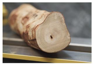
Evaluate limb; Pith must be off-center to the same side of the limb for the entire length of the limb. Pith cannot be in the center or cross through center as this will cause the stem to break. Decide which end you would like as the top of the goblet. This limb was similar in shape at both ends, but I will generally choose the more unsual shaped end for the top.
