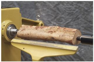
Place limb between centers with the end you decided on as the top at the headstock. Center the limb with the drive-center and live-center more or less on the center of the limb, this should position the pith out of the centerline of the goblet stem. Before turning the lathe on **sharpen your gouge**, then set the pulleys or the speed control to a slow speed before starting the lathe.
