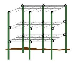
First, drive the posts into the ground in two parallel lines of three posts each. There should be 42 inches of space on either side of each row's middle post, and 42 inches of space between each row. Use the cable ties to attach the concrete remesh horizontally to the inside of the posts to form three remesh "shelves." Leave about 18 to 24 inches of height between each remesh shelf. After assembling the tomato cage, plant
