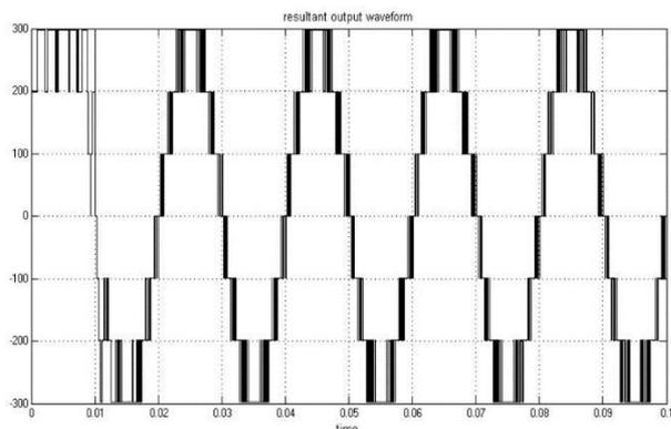
Fig. 5 Seven level Resultant output voltage waveform
