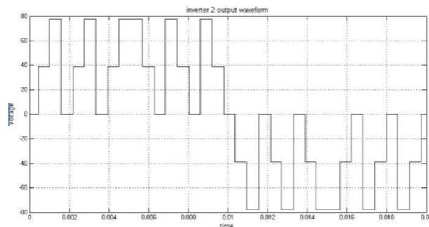
Fig. 12 Inverter 2 resultant output voltage waveform
