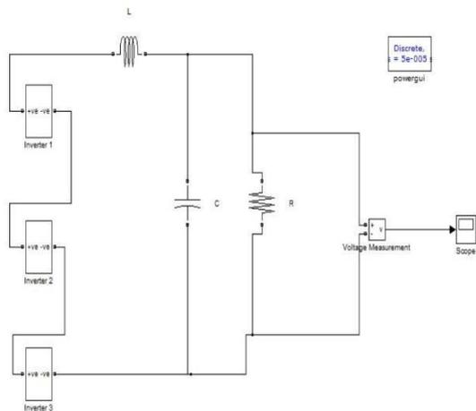
Fig. 10 Simulink diagram of newly proposed system
