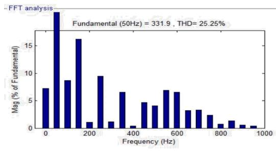
Fig. 16 THD of existing system with LC filter
