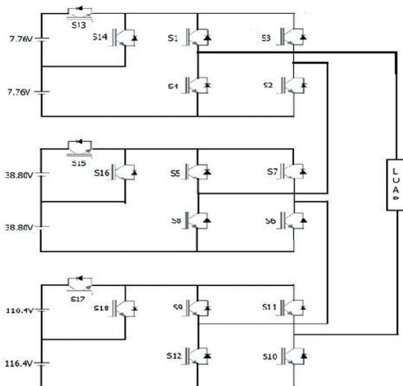
Fig. 3 Newly proposed 85 level Asymmetric multi-cell CMLI
