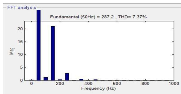
Fig. 18 THD of proposed system with LC filter
