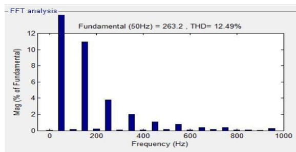
Fig. 17 THD of proposed system without LC filter
