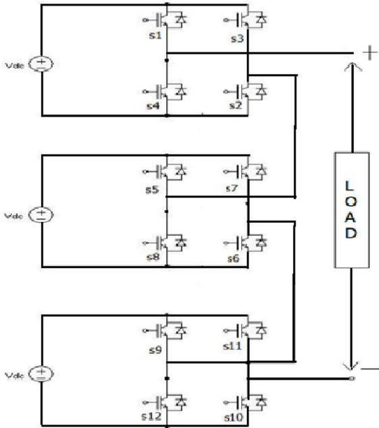
Fig. 1 Seven level inverter block diagram
