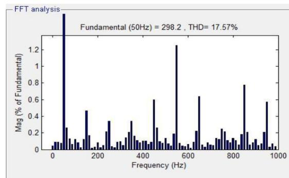
Fig. 15 THD of existing system without LC filter
