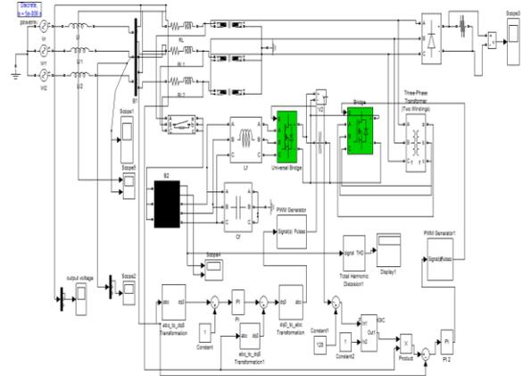
Fig.7 Simulation circuit of APF with fuzzy logic based control
