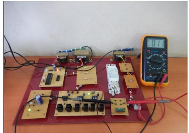
Fig.17 Prototype with the Sag voltage
