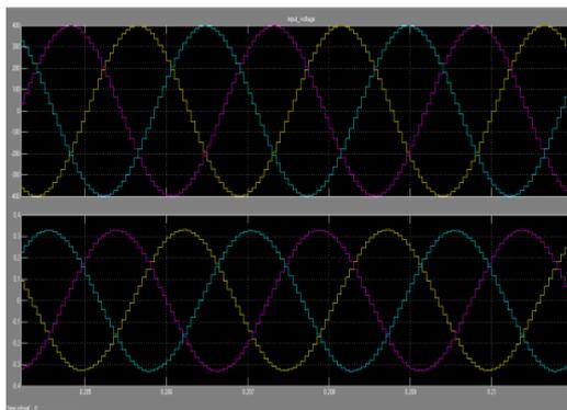
Fig.10 Source current of aircraft system with fuzzy based APF.
