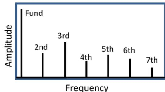
Fig.3 Typical harmonic content of an amplifier's output
