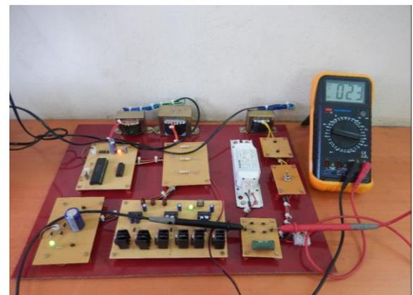
Fig.19 Prototype with the compensated voltage
