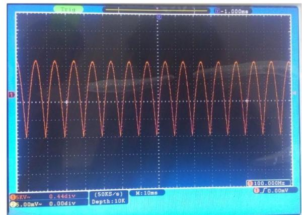
Fig.18 Digital CRO waveform of Sag voltage.
