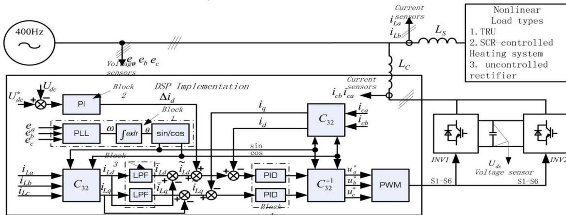
Fig.2 Structure of Active Power Filter
