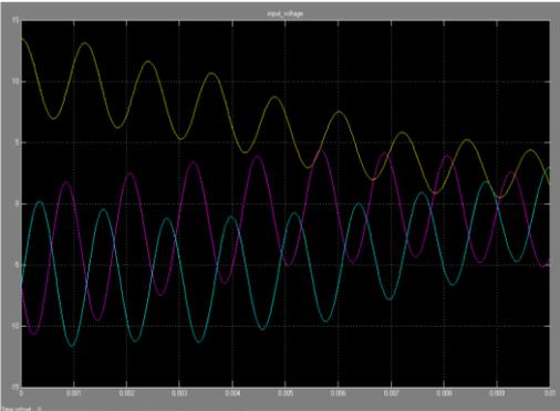
Fig.9 Source Current Without Active Power Filter
