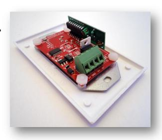
A serial interfaced FM (frequency modulation) controller for varying the intensity of a single zone of solid-state lighting. Operation and control by standard push buttons or optional RF remote control.
