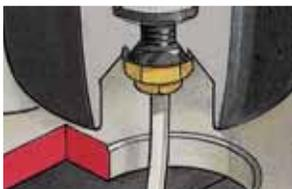
Positive removal of prefilter condensate by piping away for remote collection.
