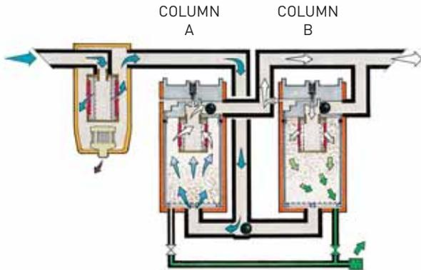
**2** Prior to changeover, the right hand chamber (Column B) enters repressurization where the exhaust valve is closed to allow pressure to increase. This process ensures a smooth uninterrupted changeover, preventing the loss of any system pressure, before the process repeats itself.
