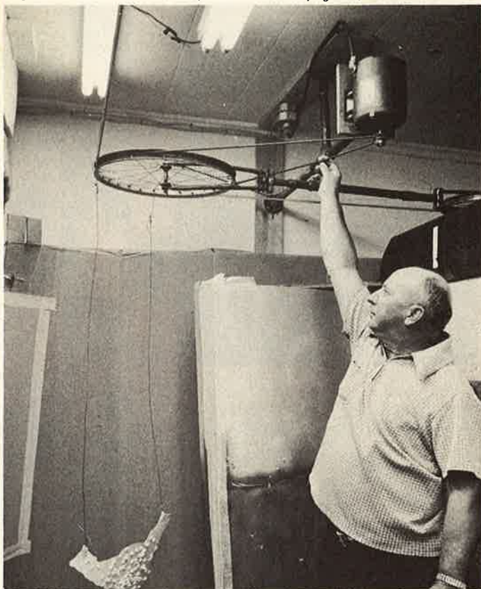
●Leo Baldwin checks the tautness of the drive belt on his indoor running game target system. Old bicycle wheels and their support brackets make excellent corner pulley units.
