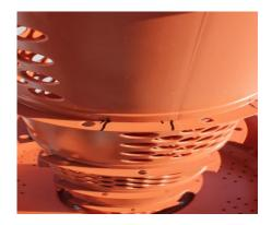
3. Now take one of the AquaJet sticks and hold it straight up and down right over one of the legs and against the center column just like in the fig below. Now with a marker or sharpie make a mark on each ledge of the tower column on both sides of the AquaJet.
