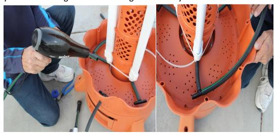
13. After the first hose is on make sure the AquaJet is still pointing over the leg and then measure the length to cut using your thumb to mark the spot where the last ridge on the barb and the hose meet. Once again make sure both AquaJets are straight over the legs before you make the cut.
