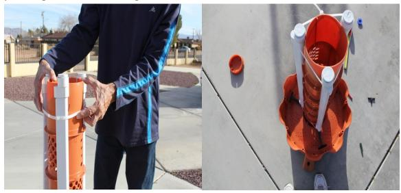
10. Now you need to drill a hole in the bottom tower for the ½ hose to go through. First drill a pilot hole 1½ inches from the bottom of the ring. See picture below. Then drill a larger hole using a 5/8 drill bit. Work the drill bit around the hole to make it easier for the hose to fit through.
