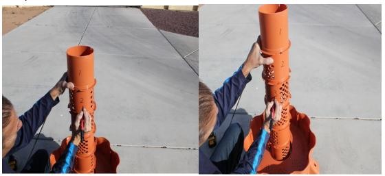
**5.** Now take some snips or wire cutters and cut out the notch that you marked on each center ring. There will be 3 notches per ring. See below.
