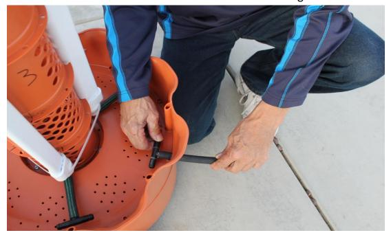
12. Now connect the hose from one AquaJet to another by first attaching the ½ in hose. If you use a blow dryer or hot water to heat up the end of the hose it is a lot easier to put on. Work the hose back and forth as you apply pressure. After you get it started you can actually turn the hose like you are screwing it on and it will go all the way down.
