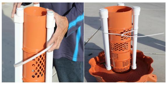
8. Now place the other zip tie around the bottom adapter (On the round part of the adapter not the oval part) and tighten snugly
