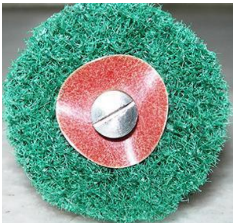
Figure 1: Rotary abrasive wheel fabricated from scouring pads
