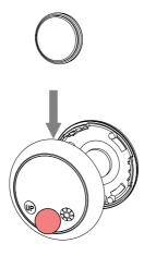
To check which mode the sensor is currently in, press the **UP** or **P2** button briefly.
