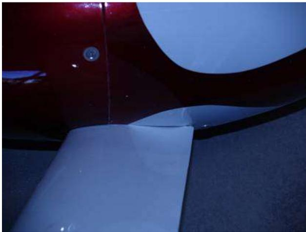
I like the fit and the fairing is very secure. Originally I had made the fit very tight causing the wheel pants to slightly bend with pressure against the fairing. Rubbing is not good as it turns into holes so I took off the pressure and gave some clearance for movement. Let you know if it works.
