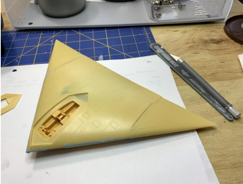
Fig. 3. Multiple applications of putty were required on every joint
