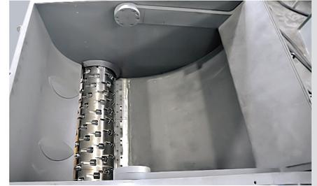
The internal ram design on the ZIS series allows the cutting chamber volume to be increased while keeping a small footprint. The ZIS is ideal for shredding of big volume parts.
