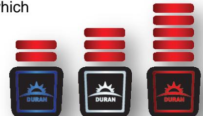
Push the button again to put the jacket in HIGH (LED button will light up solid red). Push again to go to MEDIUM heat (LED button will light up white). Push again to go to LOW heat (LED button will light up blue). Push again and the jacket will go back to HIGH. To switch off Heating, hold the button down for 3 seconds and the lighting will go off completely.
