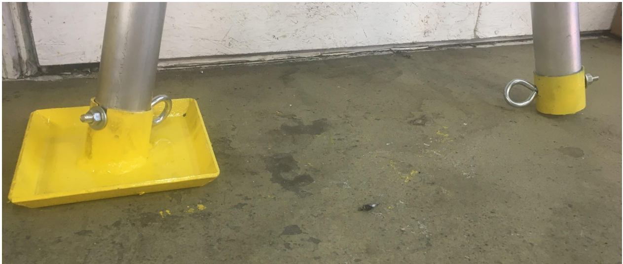
Foot Pad on left replaces Foot Cap on right..
