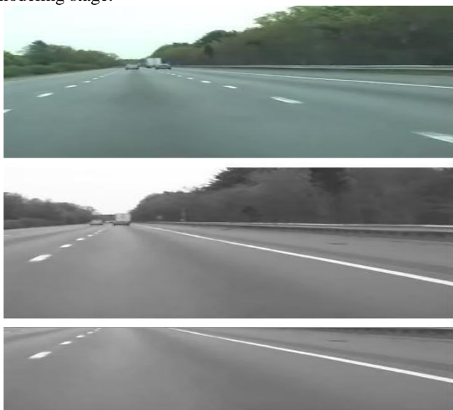
Fig.1: In the preprocessing stage, Original Image (top) is converted into gray scale image (middle). Then the region of interest is reduced focusing on the road to reduce computational time (bottom).
