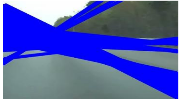
Fig.3: Reduced Resolution Algorithm detects relevant lines representing left and right lane markers.
