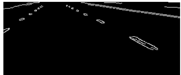
Fig.2: Canny edge detection to extract features of the lane marker.
