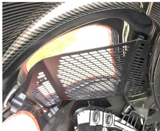
***Driver Side Shield Installed***
