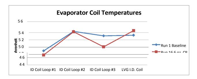
These polymers circulate with the refrigerant and when they get to the evaporator they provide inert particles that aid in nucleation during the pool boiling phase. Simply put it is like water boiling at a lower temperature when you introduce a substance like salt. This change in pool boiling will lower the evaporator temperature and allow for more efficient operation.
