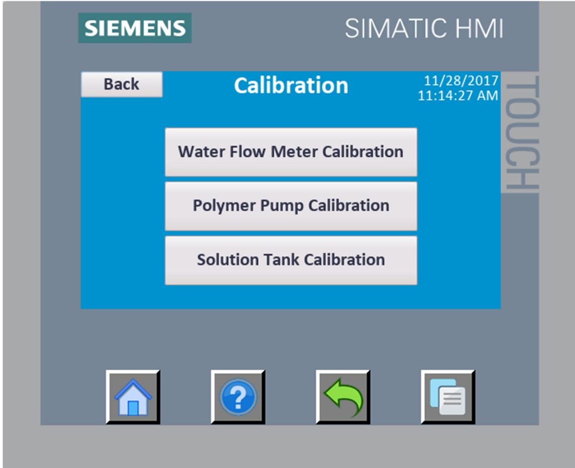
The water flow meter, polymer pump, and solution tank all have available calibration settings. Each calibration screen can be accessed by pressing their respective button.
