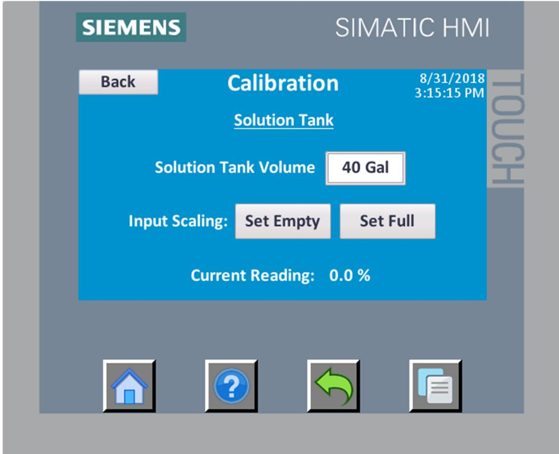
The solution tank uses a submersible pressure sensor to measure the height of liquid in the tank. If the tank level value on screen does not match the level in the tank then, then the Set 4mA and Set 20mA buttons can be used to scale the input. The correct volume at the 100% fill height must also be entered. The volume is used to calculate how much liquid it should take to fill the tank during each makedown cycle.
