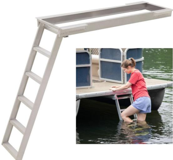
Five step Under-Deck ladder extends 59" below the deck. Rated to 300 lbs. Conveniently stows under the pontoon deck when not in use. When deployed it pulls out at an angle for easy climbing. Bolts to the cross members under the deck.
