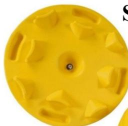
Rotationally molded plastic anchor has a smooth top to protect feet, underside has claws to grip the lake bed. Fill with sand to create a 140 lb. anchor. Has eyelet on top for connecting rope or chain.
