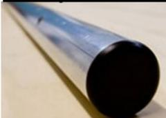
Heavy wall Aluminum pier pipe is drilled for turn bars on the top and augers on the bottom. Also capped on the top end to protect your hands. Available in 8', 10', 12' & 16' lengths.
