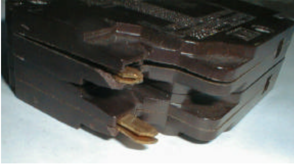
Figure 8 – Damaged “E” type breaker
