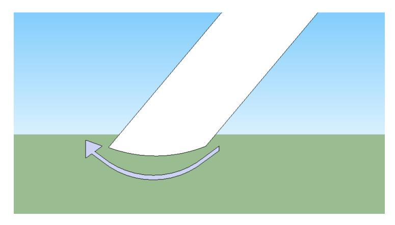
(Exaggerated hollow grind bevel) Notice that the hollow grind wants to follow a radius into the work piece.
