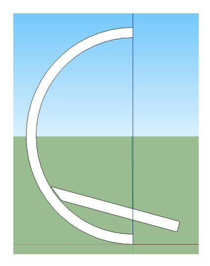
Notice how the angle of bevel is so steep it gets close to the side of the bowl, then at the bottom, the gouge runs into the side of the bowl. Now the tool is almost to the bottom of the bowl and is rubbing the side of the bowl. It can not complete the cut
