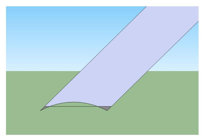
Notice that honing changes the cutting action. Instead of digging in, it will move straight ahead. It is still sharp, it just cuts (feels) different.
