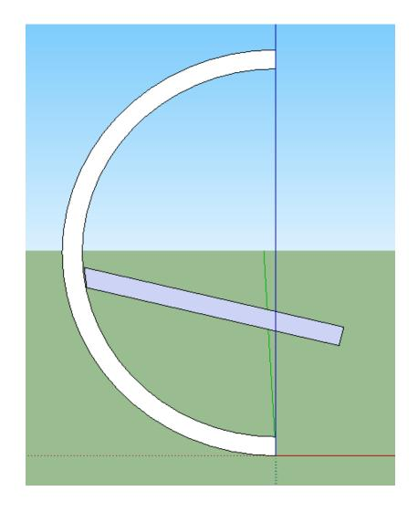
Notice that the tool clears the sides of the bowl all the way to the bottom
