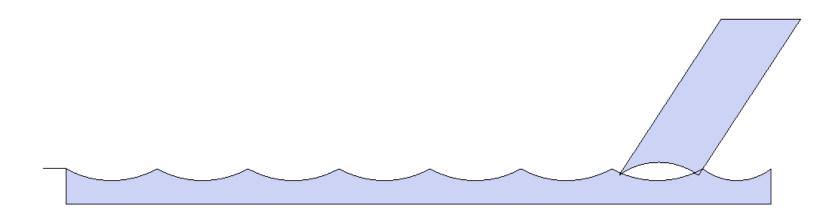
The long bevel and hollow grind will rise and fall with the washboard tool marks
