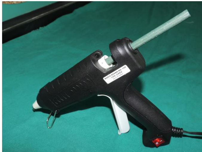
Figure 1. Modelling compound loaded in glue gun.
