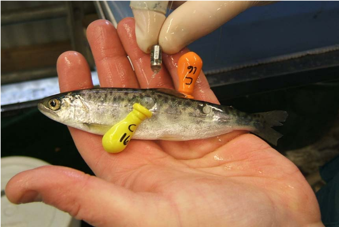
Figure 5. Juvenile Chinook equipped with two uninflated HI-Z tags and a miniature radio tag.
