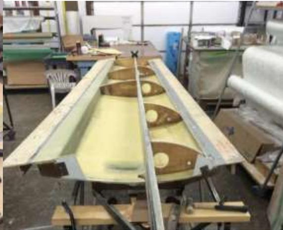
**Spar and Ribs Installed**
