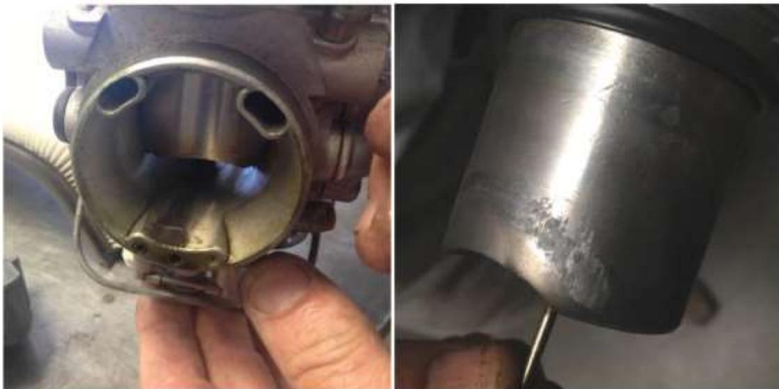
Figure 3 – Carburettor Contamination & Slide Wear
