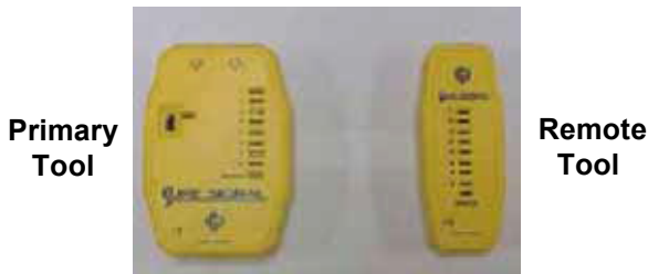
Figure 5.10 Cab Command Diagnostic Tool (CTD P/N 07-00440-00)
