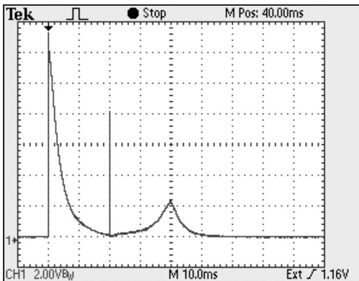
Figure 4 –  $\pi/2, \pi$  Pulses, Light Mineral Oil
