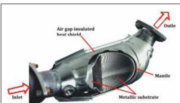
Figure 2: Structure of a metal catalytic converter
