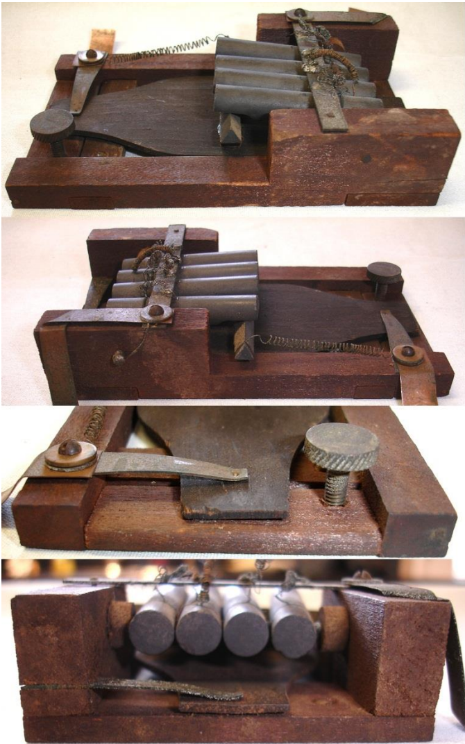
1889 Harrison International Telephone Transmitter US Patent filed 8-9-1890 & issued 5-31-1892
