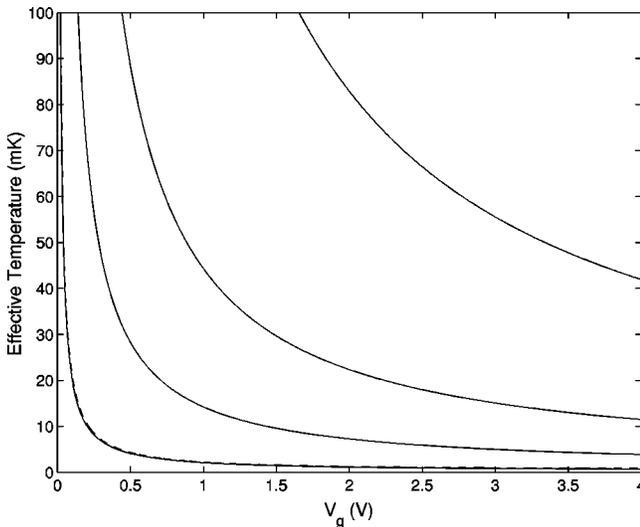
FIG. 3. Estimates for the minimum achievable effective temperatures as a function of gate voltage for a range of initial temperatures,  $T$ . On this plot, the increase in achievable temperature which results from the restriction  $k/\beta \leq 0.1$  is virtually imperceptible for  $T$  above 100 mK. For  $T=100$  mK the dotted line shows the result under this restriction. From top to bottom, the initial temperatures are 2 K, 1 K, 500 mK, and 100 mK.
