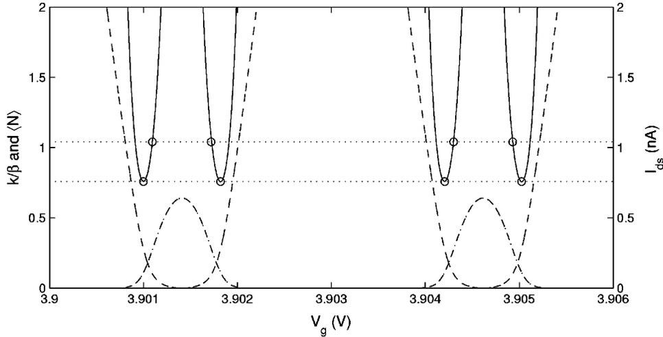
FIG. 2. The steady-state average occupation number,  $\langle N \rangle$ , as a function of the gate voltage (solid line), plotted along with the ratio  $k/\beta$  (dashed line), and the drain-source current,  $I_{ds}$ , (dot-dashed line). The lower dotted line gives the minima of  $\langle N \rangle$ , and the upper dotted line gives the values of  $\langle N \rangle$  when  $k/\beta=0.1$ .
