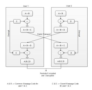
Fig. 4. Diffie-Hellman Key Exchange Method
