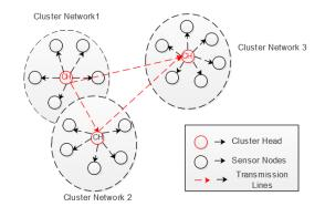
Fig. 2. Basic Clustering in Mobile ad-hoc network
