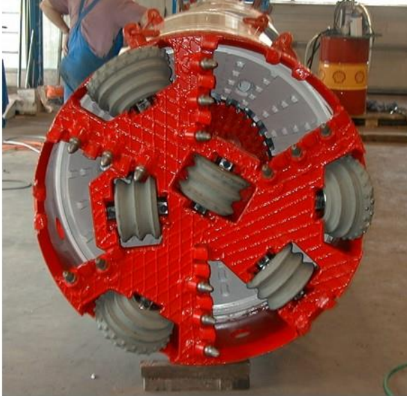
Mixed Face & Soft Ground Cutter Heads & Replacement Cutters
