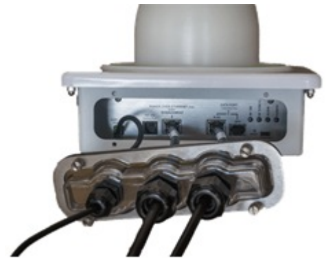
Figure 8: System backpanel and transparent cover lid
