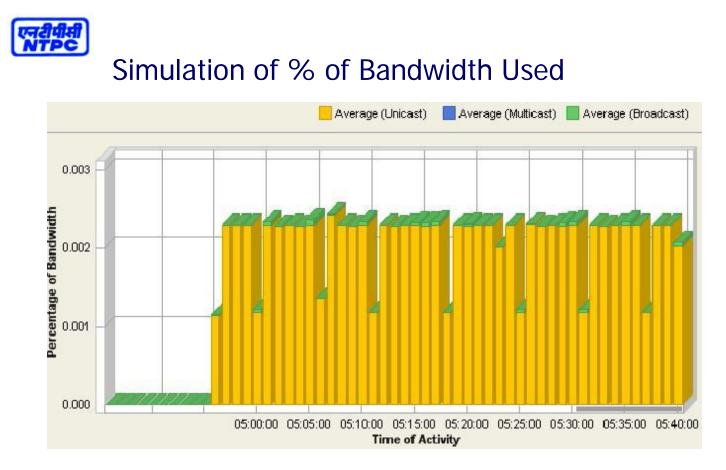
When GOOSE is enabled with a time-to-live (TTL) of 1 second, the expected result is an increase of bandwidth use, as shown above
