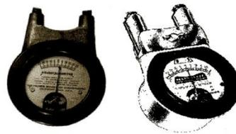
**Neurocalometers (neurocollometers) measured heat along the spine via thermocouples.**
