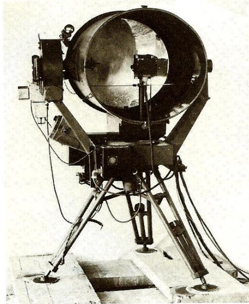
Baird Evaporograph System used by Leo Massapust in 1948
