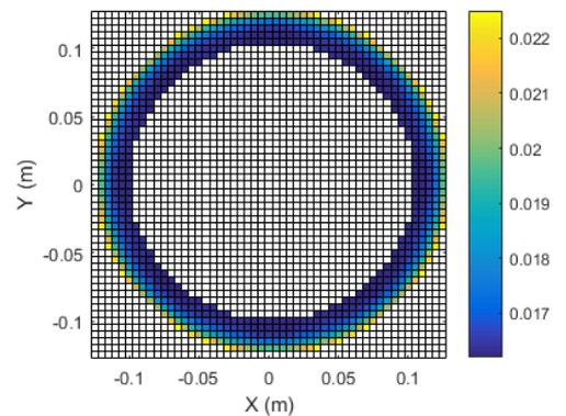
**Figure 1:** Current distribution over the cross section of the casing sample at 100 Hz.
