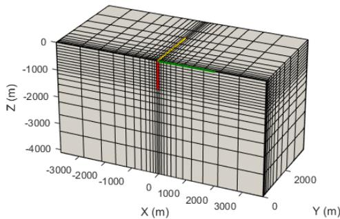
**Figure 4:** 3D mesh used in the demonstrative example. Red line: casing; yellow line: source wire; green line: receiver line.
