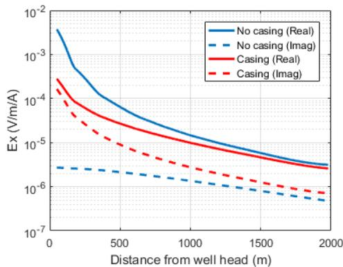
**Figure 5:** Simulated surface E-field data at 10 Hz with and without casing.
