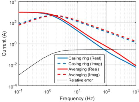
**Figure 3:** Equivalent total current in the casing sample when modelled using the actual ring shape and using a solid rod with an averaged conductivity.
