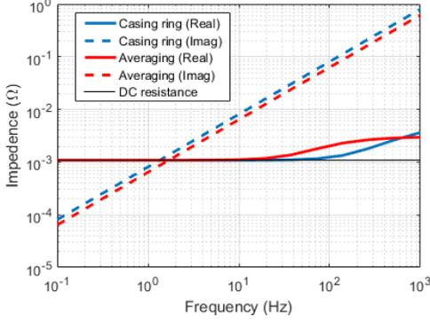
**Figure 2:** Equivalent impedance of the casing sample when modelled using the actual ring shape and using an averaged resistivity.
