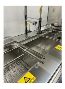
2 stainless steel (316 grade) ultrasonic tanks with agitation arm
