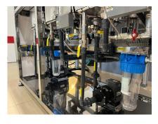
Automatic detergent filtration for both US tanks. (Magnetic Pump Circulation)
