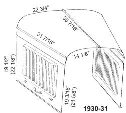
Measurements in parenthesis are for 1930-31 3 piece hood.
