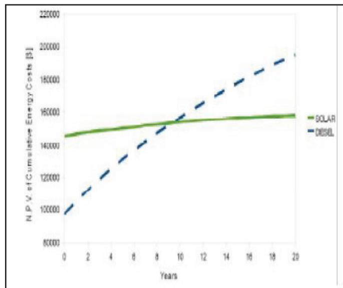
Fig. 3: Cumulative Cost of Energy System for Off-Grid Cell Site (Solar v/s Diesel) [6]
