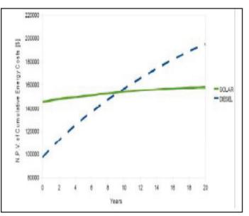
Fig. 3: Cumulative Cost of Energy System for Off-Grid Cell Site (Solar v/s Diesel [6]
