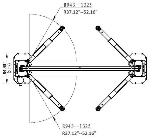
Fig. 3 (Column / Floor Layout)
