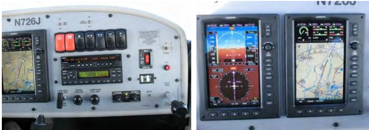
New Aveo switches on the left and the Garmin G3X system on the right.
