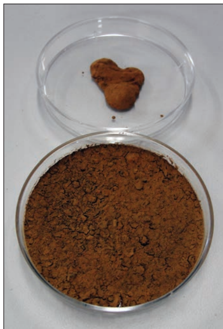
Comparing deposit samples with water analysis can help determine the extent of a problem occurring downhole.
