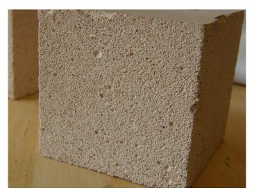
This finished product is very lightweight, **fire resistant**, insulating and provides structural support in a SIPs panel application, far in excess of what might be provided from a conventional Expanded Poly Styrene (EPS) core.
