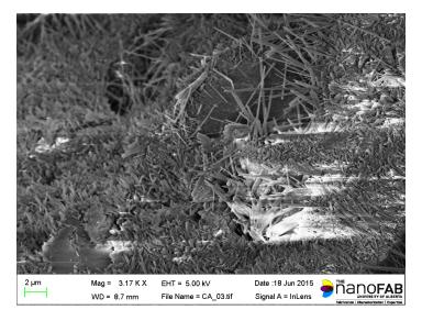
The image above shows the results of an SEM image of the final product magnified several thousand times. The long tubular structures accounts for its very high strength.
