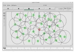
Fig. 5: Nodes exchanging Hello packets
