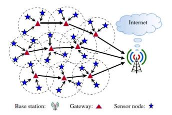
Fig. 1: A Wireless sensor network model
